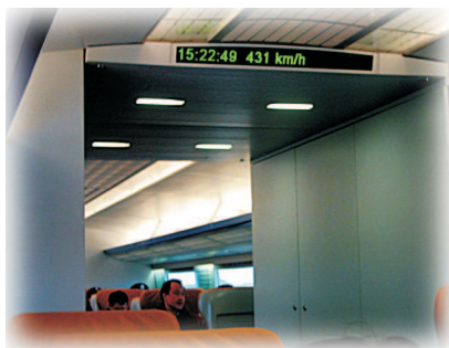
Custom-made passenger info displays for the Transrapid trains to Shanghai 100mm char., length 2-8m, for the CEBIT-exhibition/Germany
