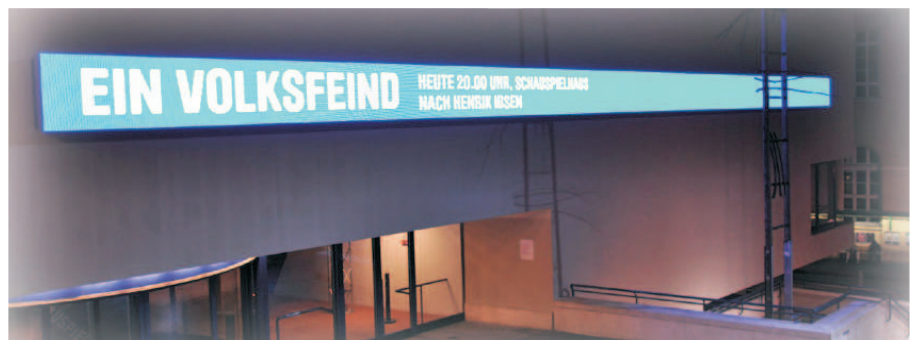
Basel theatre: 23,5 x 1m facade-videodisplay with SMD 3in1 outdoor leds, front-maintenance
