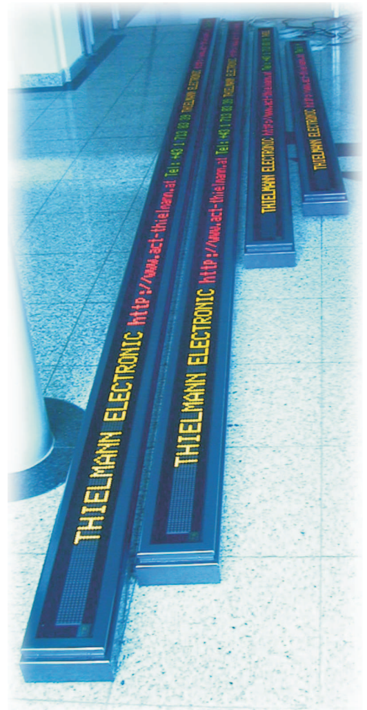
Custom-made passenger info displays for the Transrapid trains to Shanghai 100mm char., length 2-8m, for the CEBIT-exhibition/Germany
