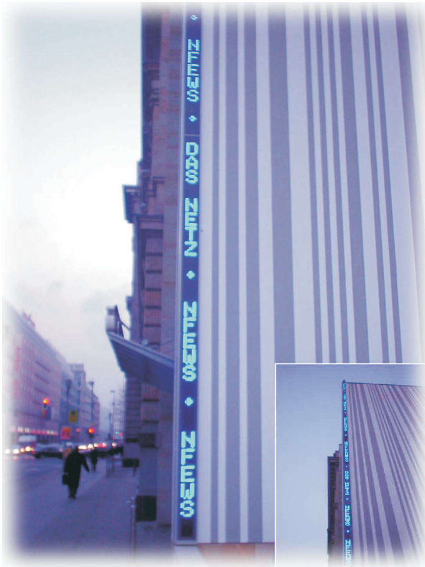
Europeans longest led-pillar with blue leds, 21m high, 200mm char., mounted in Berlin/Germany
