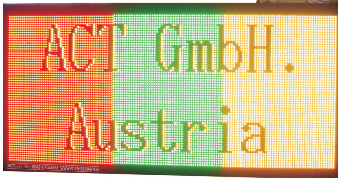
2,4 x 1,2m graphic display with 16mm pixel pitch
