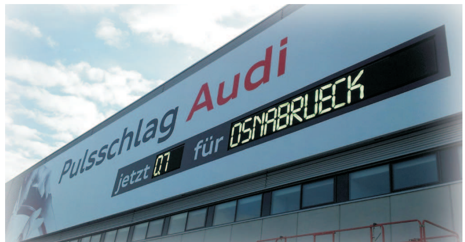
130.000 ultrabright flat-leds: 18x1,3m for info / advertising, car production plant AUDI-Ingolstadt
